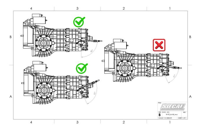
The shift linkage and cable should be set up to be 90 degrees from the center of the shift linkage pivot center and the cable, as shown above. Not having the linkage properly configured will lead to a shift travel that is not centered at the shifter, overtravel of the cable, difficulty in making smooth shifts, and in some cases, damage to the transmission.
