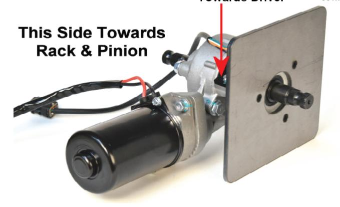
NOTE: The red and black wires must go directly to the battery. Do <u>NOT</u> wire the computer to your fuse box. Wiring the computer to the fuse box allows for a short voltage drop that turns the unit off intermittently. Do <u>NOT</u> cut the wires that lead from the computer to the motor. Any alterations to those wires voids any warranty.
